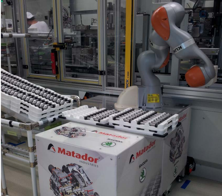
Fig. 2 – Collaborative robot integrated in ŠKODA AUTO a.s. Vrchlabí (Czech Republic)
