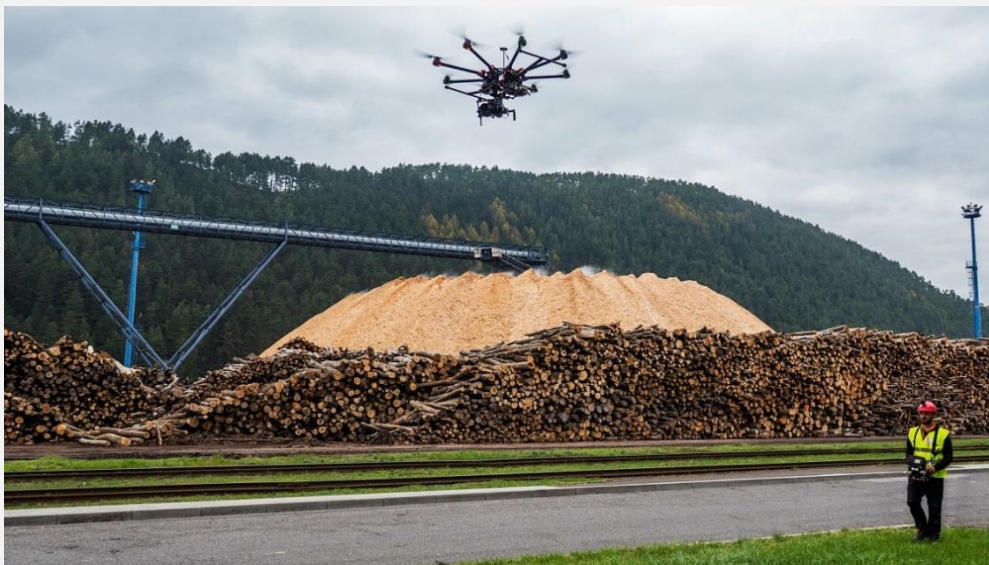
Fig. 6 – Volumetric Measurements by UAV
