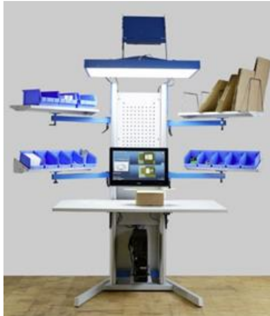
Figure 63 Work instructions are projected on assembly table 13
